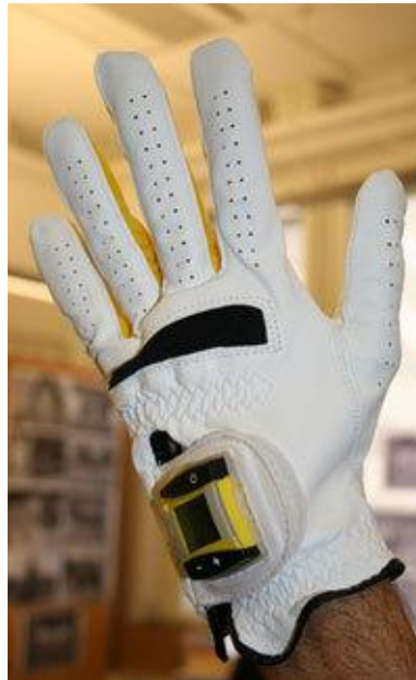
Figure 1: A pressure sensing golf glove designed to provide real-time feedback on club grip pressure.
